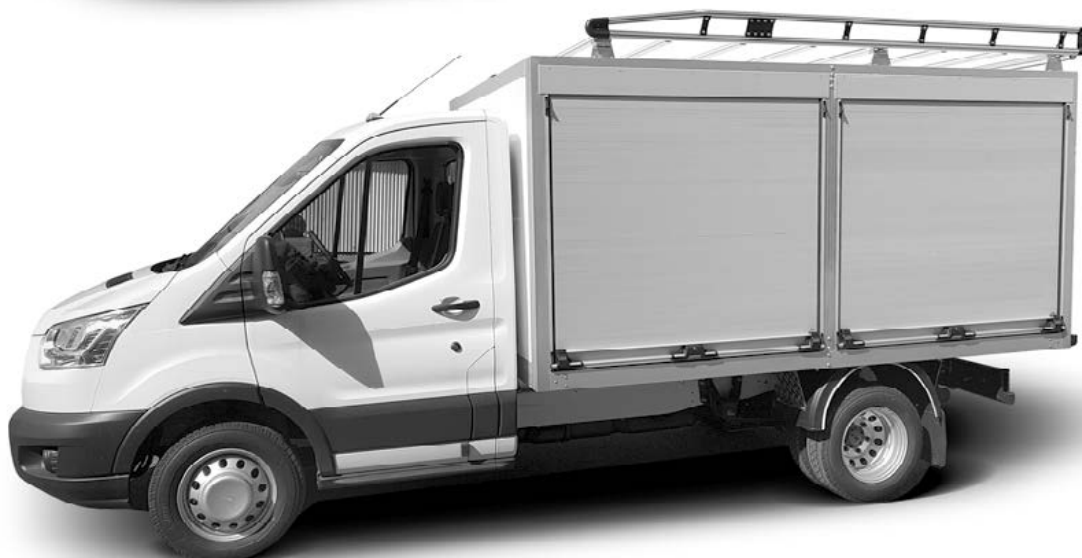
Rolety s navíjením na buben ( po stranách ) a pod střechu (vzadu ) Shutter with winding on balancer ( on the sides ) and with winding under the roof (at the back)
